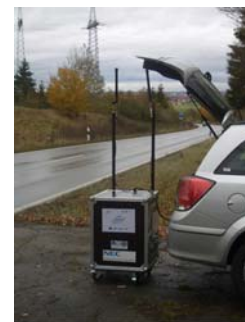
Road Side Unit with construction site warning
